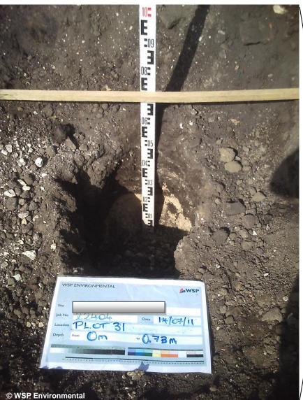
Photograph 2: Depth check of inert cover with Site & Location Information Board.
